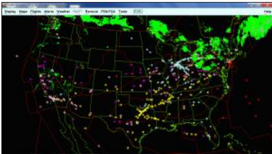
Fig. 1.1 – As a part of the Traffic Flow Management System (TFMS), the Traffic Situation Display (TSD) allows the traffic management specialist to graphically display the current position of all instrument flight rule (IFR) flights that are in the air. The software has the functionality which allows the Traffic Manager to graphically display future demand as well.
